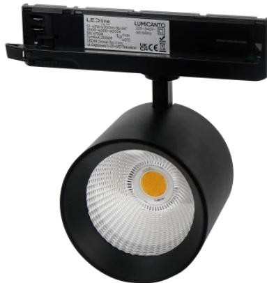
Track light LUMICANTO 6-20W CCT 36/60° in black, is a modern LED line PRIME lighting setting. It uses innovative COB-Bridgelux diodes, characterized by high light performance of up to 110 lm/W and variable colour temperature: 3000 K, 4000 K and 6000 K. The luminaire provides excellent colour reproduction ( $R_a \geq 90$ ) and a low flickering factor. With IP20 and IK06 certifications, it offers reliability in different conditions, and its durability is as high as 50,000 hours.
