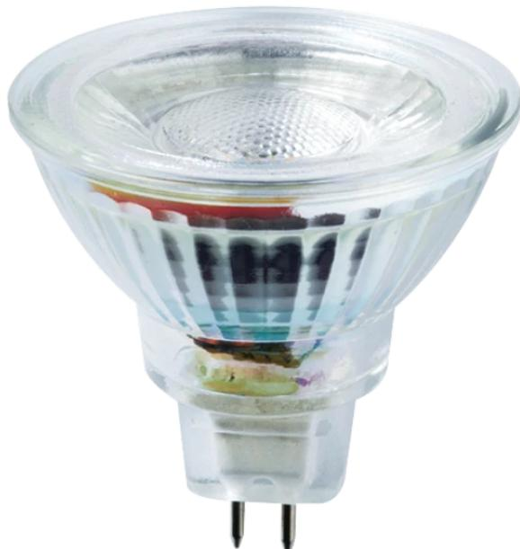
LED line bulb LITE MR16 3W with warm light color 2700K emits a light stream of 273 lumens, which provides a cozy atmosphere. Powered by a voltage of 10-14V AC/DC, it has a light output of 91 lm/W and a long service life of up to 30,000 hours. Thanks to a light angle of 36°, it is ideal as point accent lighting. SMD2835 Diodes guarantee stability and lack of flickering effect, eliminating eye fatigue.
