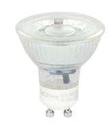
LED line bulb LITE GU10 5W 2700K is an energy-efficient light source with a light stream of 410 lumens. It is characterized by warm white colour, creating a pleasant mood. At 5W, it achieves high light performance at 82 lm/W and Ra  $\geq\!80$  color reproduction coefficient, providing natural color reproduction. With a shelf life of up to 30,000 hours and resistance to 50,000 on/off cycles, it is a reliable solution.
