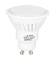
LED bulb GU10 10W 2700K 1250Im from LED line PRIME is an innovative light source, characterized by high light efficiency of 125 Im/W. Thanks to the use of SMD2835 diode technology, the product generates a pleasant, warm white light with a colour temperature of 2700 K. Powered in the 170-250 V AC voltage range, it offers a long life of up to 30,000 hours and the ability to adjust brightness with compatible TRIAC dimmers.
