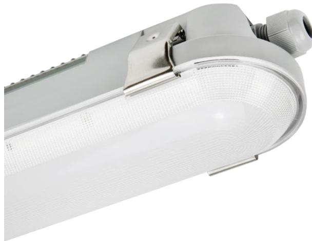
LED line RANGER C 40W is a modern hermetic lamp with a high luminous efficiency of 140 lm/W. At a power of 40 W, it generates a luminous flux of up to 5600 lm, providing excellent lighting at a color temperature of 4000 K. The product features an IP66 ingress protection rating, ensuring resistance to dust and water as well as mechanical damage (IK08).
